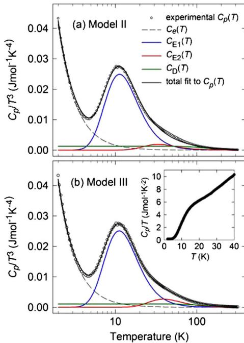
FIG. 1 (color online). Specific heat capacity of  $\text{Na}_{24}\text{Si}_{136}$  plotted as  $C_p/T^3$  against  $T$ , along with fits obtained with (a) Model II and (b) Model III described in Table I. Individual contributions to the overall fit are also shown as indicated. Inset to (b): The same experimental  $C_p$  data plotted as  $C_p/T$  against  $T$ , in the temperature range 0 to 40 K.
