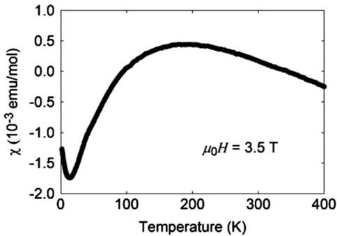
FIG. 2. Magnetic susceptibility of Na<sub>24</sub>Si<sub>136</sub>, measured in an applied field  $\mu_0 H = 3.5$  T.
