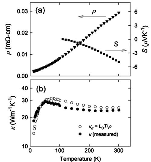
FIG. 3. (a) Electrical resistivity ( $\rho$ ) and Seebeck coefficient ( $S$ ) of Na<sub>24</sub>Si<sub>136</sub>. (b) Thermal conductivity ( $\kappa$ ) of Na<sub>24</sub>Si<sub>136</sub> (closed symbols) and calculated contribution (open symbols) estimated from the Wiedemann-Franz relation.
